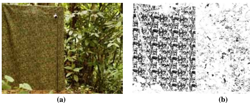
Figure 1: (a) A typical experimental setup involving a textile material hung vertically in a forest environment. In the centre of the image is the Spyder colour calibration cube hung on a thin pole. (b) A binary image formed by selecting Lab values of a specific dye (green in this case) on the textile. The same values of Lab also selected similar green colours in the background. The regularity of pattern caused by the printing process is seen on the textile, but the corresponding leaves in the environment are random.
