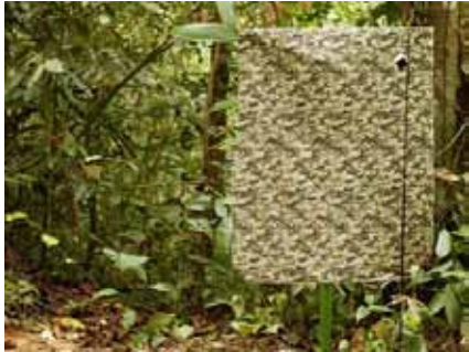
Figure 3: Colour photograph of a camouflage textile against the background forest. This material was made with generally lighter colours.
