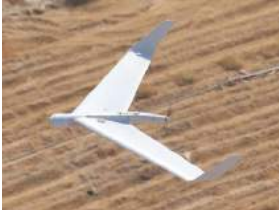
Figure 3: Aeronautics' Orbiter IK UAV, which can carry up to 2 kg of explosives in its fuselage.
