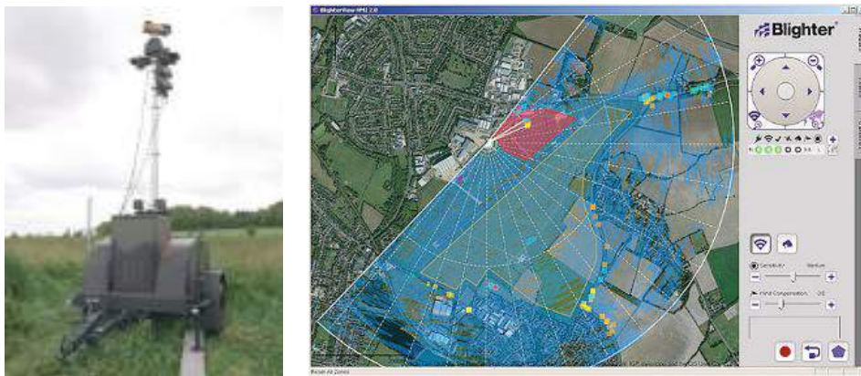
Figure 8: The Blighter radar system developed by Plextek for detection of UAVs. (Source: Baker) [35]
