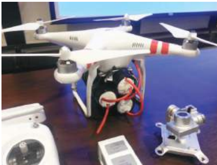
Figure 2: A UAV equipped with 3 lbs of mock explosive. (Source: Poulsen) [17]
