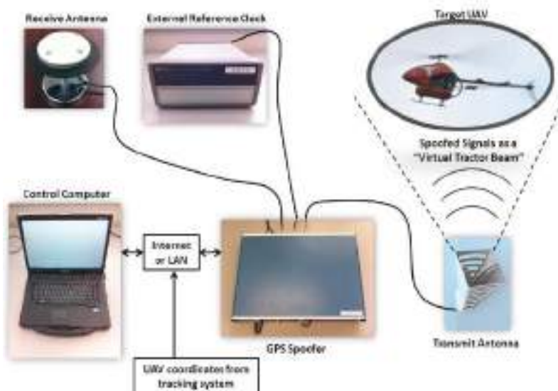
Figure 14: Global Positioning System (GPS) spoofing conducted by Shephard et al. [31].
