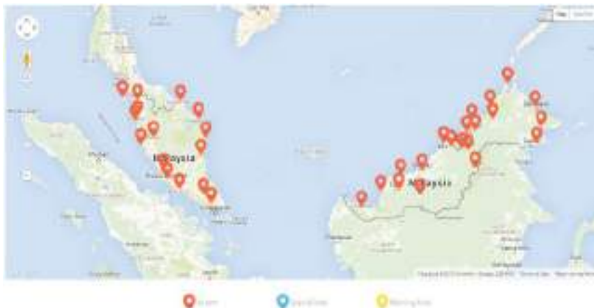
Figure 7: Exclusion zones for Malaysia set in DJI's geofencing software. (Source: DJI) [14]
