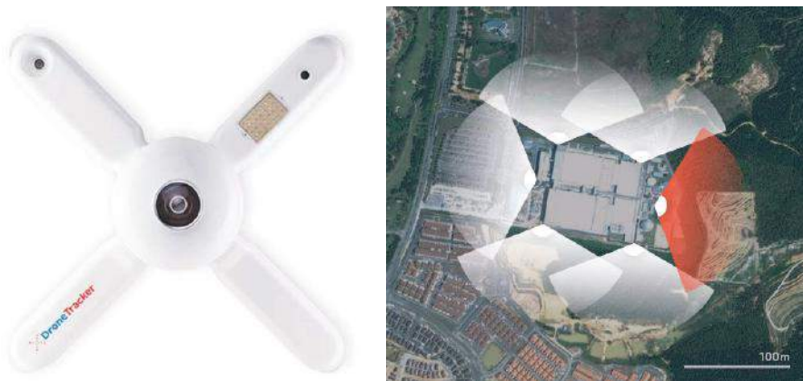
Figure 12: Dedrone's DroneTracker can be used to form an EO sensing network. (Source: Dedrone) (2015))
