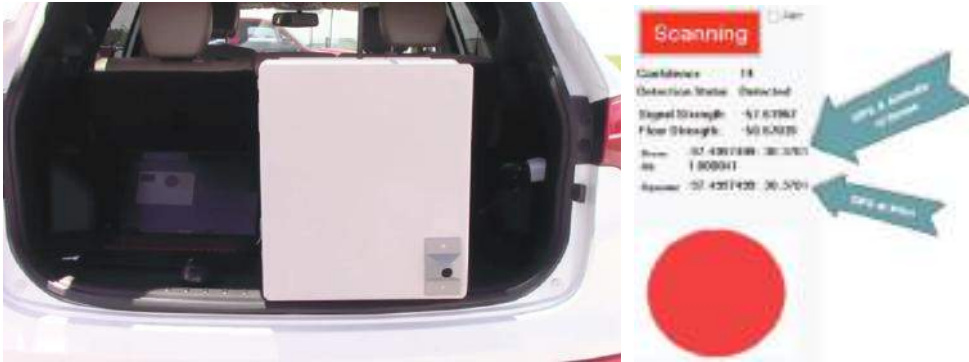
Figure 11: Drone Labs' DD610AR RF emission sensing system for detection of UAVs. (Source: Drone Labs) [38]
