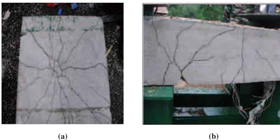
Figure 8. Damage pattern of the NRC panel.
