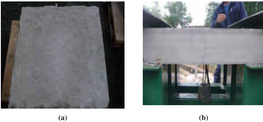
Figure 9. Damage pattern of the HSFRC panel.
