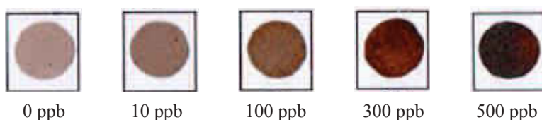
Figure 1: Arsenic standard colour chart in ppb.
