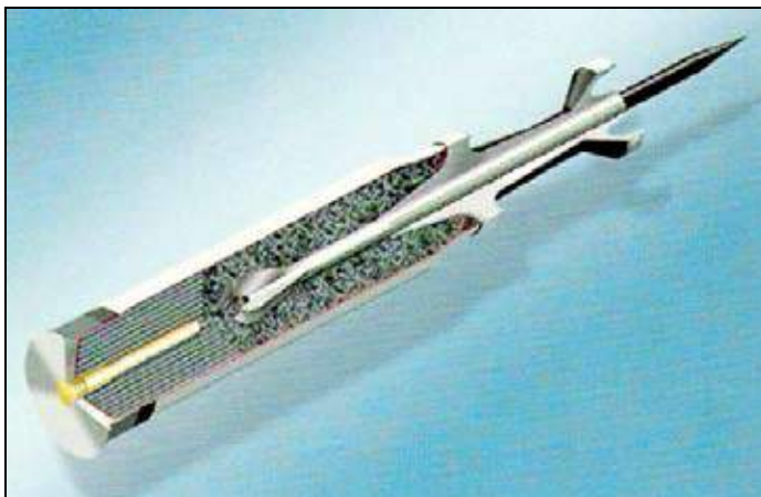
Figure 1: A cutout diagram of a Fin Stabilized Discarding Sabot [22]
